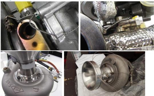
Examples of incorrect sealing wiring
